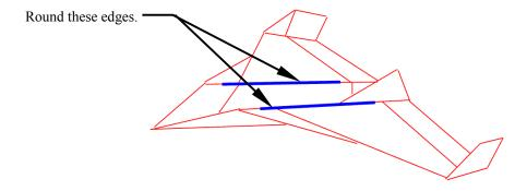
The next part to adjusting is to get straight and level flight. If the nose is going down or plane just doesn't have enough lift then curve back (trailing) edge of wing up as shown. If nose goes up then curve trailing edge down. For both of these adjustments, you may have to make curved edges and then straighten back as good as you can while leaving just a very slight adjustment.
