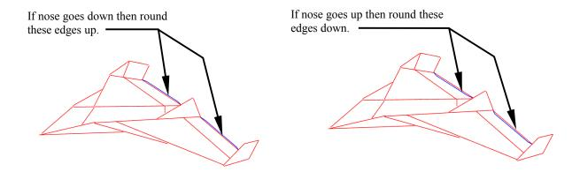
If the plane has a tendency to flip over and fly upside down, then try folding the fins to the opposite side, or add fins if there are none. Adding or removing the tail can become necessary when going from one type of paper to another. Adding a tail will bring the nose up and removing one will bring the nose down. If the plane spins out of control, then make sure that the wings are angled up, not down. This angle is called dihedral angle and is important for stability (helps prevent rolling).
