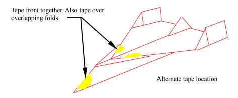
If you don't tape then you will have to smooth out some of the edges. Air does not like to flow over or across sharp corners. This can cause the plane to want to spin to one side or the other if you don't round the edges between the body and the wings as shown below.
